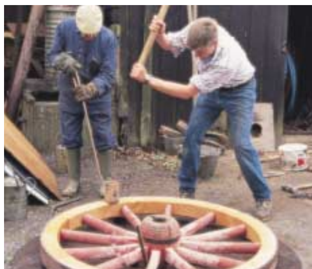
Wheelwright Douglas Andrew hammering rim into position
