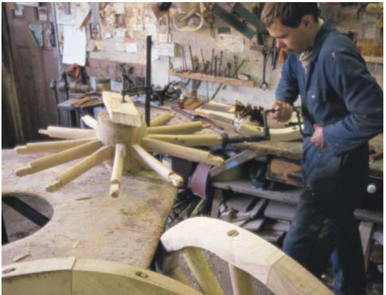
Using brace and bit to finish spokes
