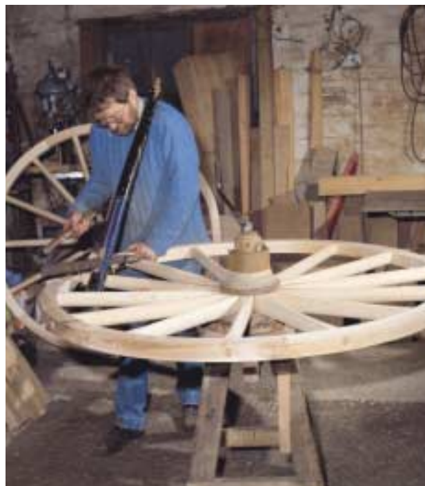
Using a spoke-dog to fit a fellow
