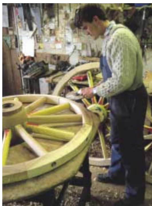
Wheelwright measuring rim with traveller, Sussex
