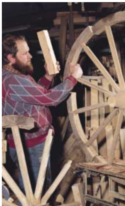
Wheelwright hammering felloes onto spokes, Devon
