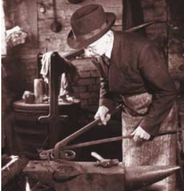
Blacksmith forging iron scroll (1930s)
